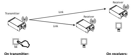
Press the Link button to link all unlinked receivers in the range of the transmitter.
