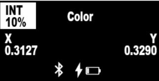
Color mixing via CIE 1931 xy is available via the myMIX app. This function is not available via the onboard interface, however, the xy settings chosen via the app will appear on the Active Screen while being controlled via the app.
