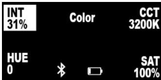
Color Mode is for creating custom colors using HSI (Hue, Saturation and Intensity). Use the Navigation Button to select an attribute to modify.
