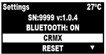
Press the Navigation Button or rotate the Dimming & Selection Wheel to highlight the CRMX option.
