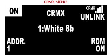
Use the Navigation Button to select an attribute to modify, then press the Dimming & Selection Wheel to access the desired attribute.
